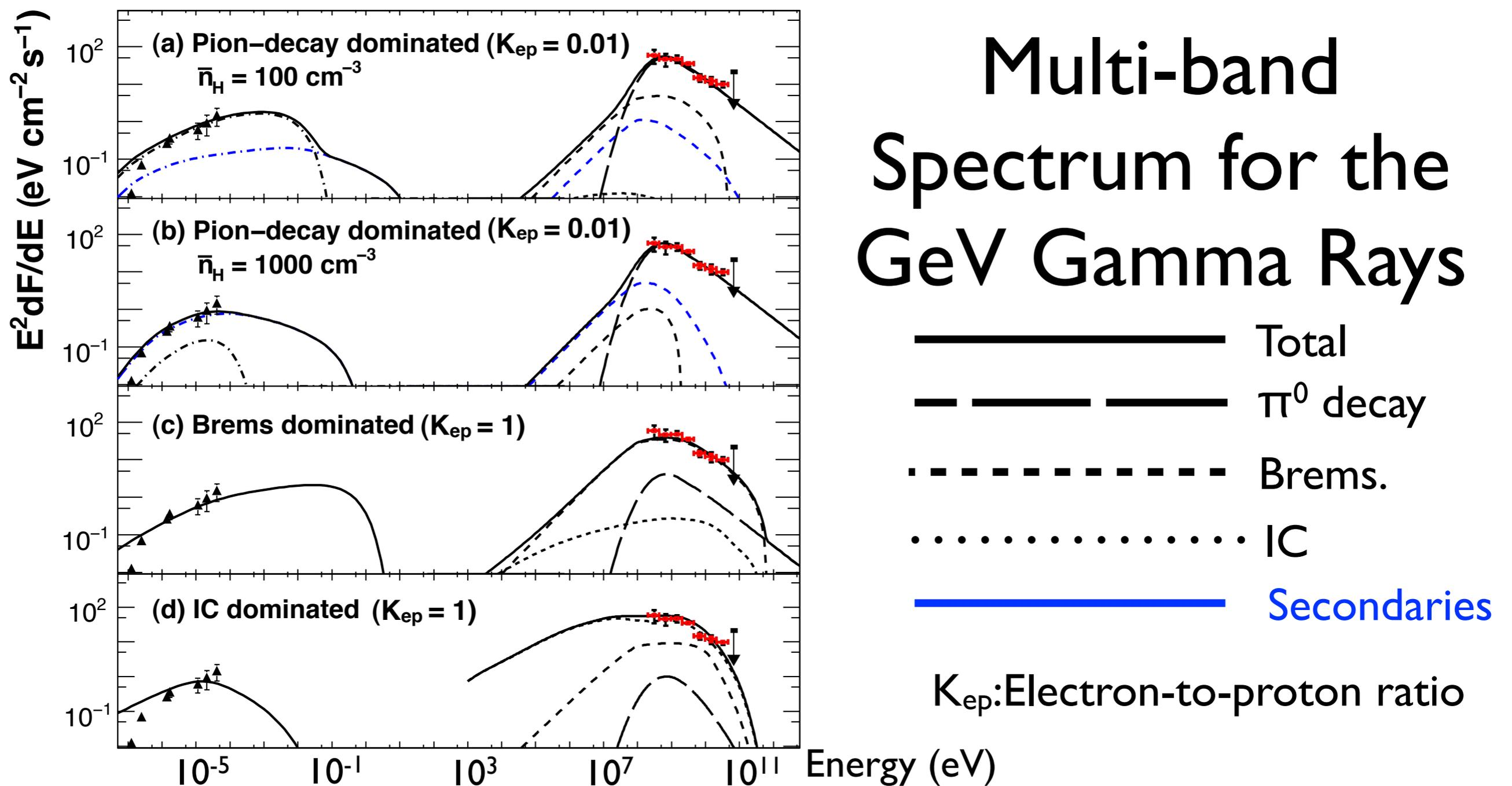
■ The GeV gamma-ray spectrum is naturally explained by  $\pi^0$  decay produced by the interaction of the MCs and particles accelerated by G8.7-0.1.
