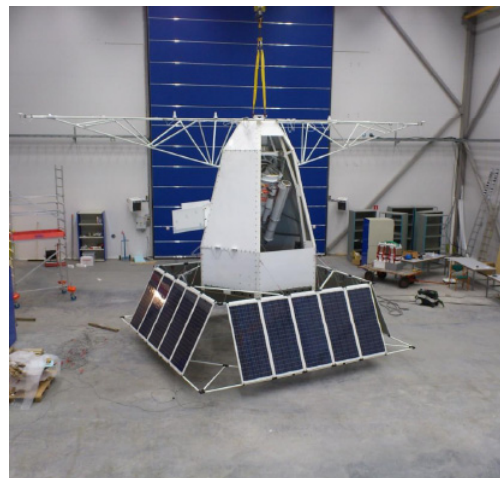
PoGOLite (2012) 30-80 keV balloon, Plastic scint.
