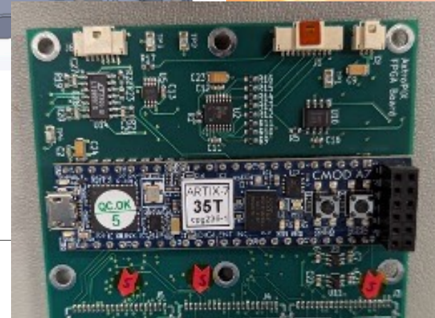
Front-end electronics + flight computer
