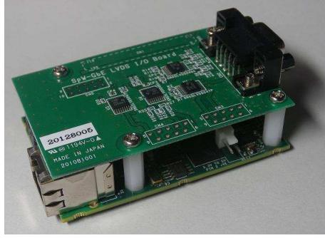
図 2.15: SpaceWire Gigabit Ethernet
