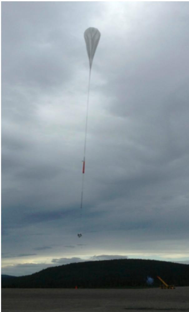
Figure. 2.1: The launch of PoGOLite from Esrance on July 12th 2013, 0818 UT. The distance from the top of the balloon to the gondola is  $\sim 300$  m.
