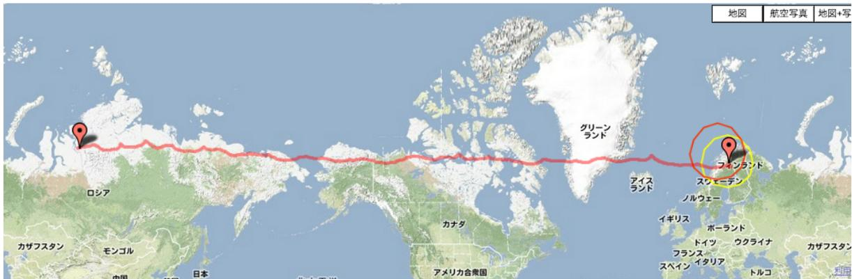
Figure. 4.1: The trajectory of PoGOLite after the launch from ESRANGE. The tendency for the balloon to follow a Northerly track is seen in the days prior to termination. The launch took place from ESRANGE on 12th July at 0818 UT and the gondola landed in Siberia on July 25th at 0015 UT. In the yellow and red circles, E-Link communications are available.
