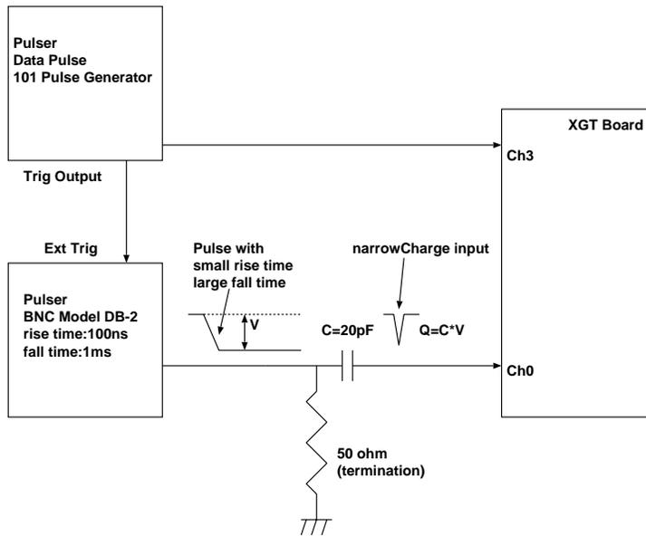
Figure 2: Setup to collect data for small charge input.
