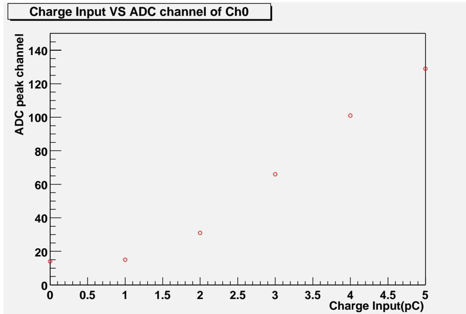
Figure 4: Relation between ADC peak channel and inputted charge of Channel 0, when the amount of charge is quite low.
