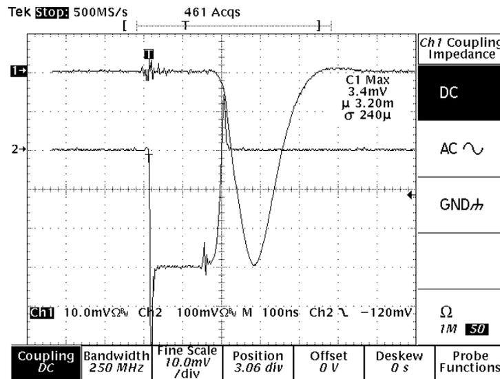
Figure 3: Voltage pulse put into Channel 3 (trace 2) and charge pulse put into Channel 0 (trace 1), both in 100 ns/div. The former hit the low-level discriminator, and starts DAQ system. Since the latter signal comes into XGT board almost at the same time, we can collect histogram of this signal simultaneously.
