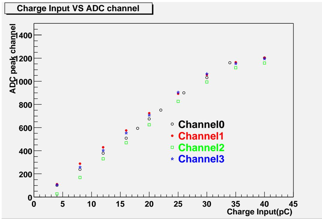
Figure 1: Measurement of gain and offset of XGT board. ADC peak channels are plotted as a function of the amount of injected charge.
